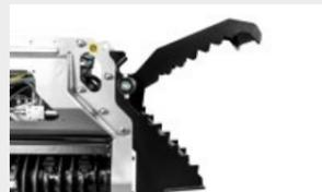
**Thumb bracket and hydraulic thumb**
